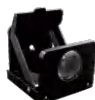
Microhole (4mm) transmission test fixture assembly Make sure the petri dish is fixed for measurement.
